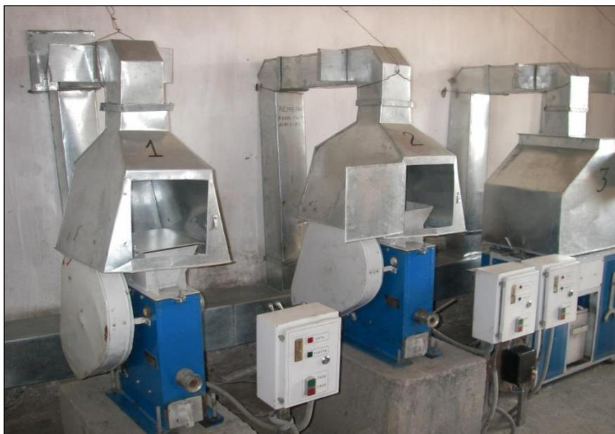
**Figure 4-18: Sample Preparation – Crushing Equipment**
