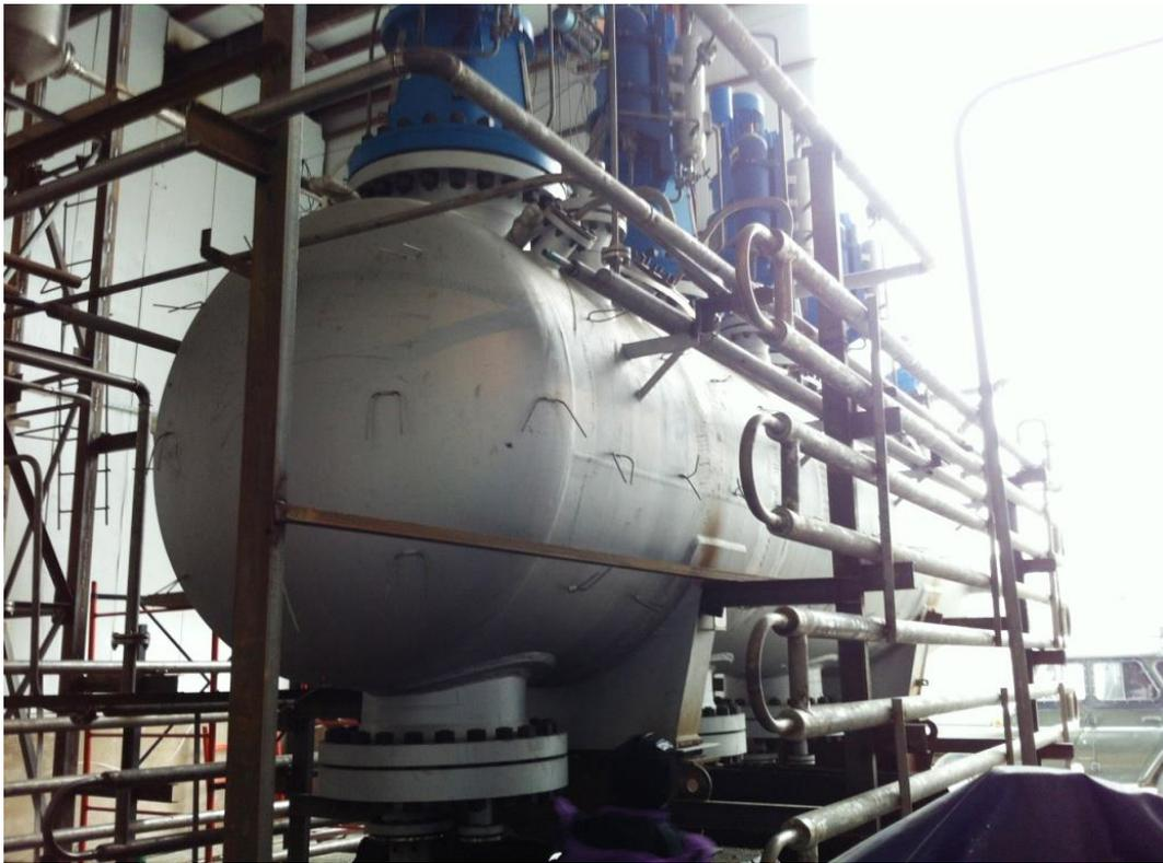
**Figure 7-5: Autoclave**
