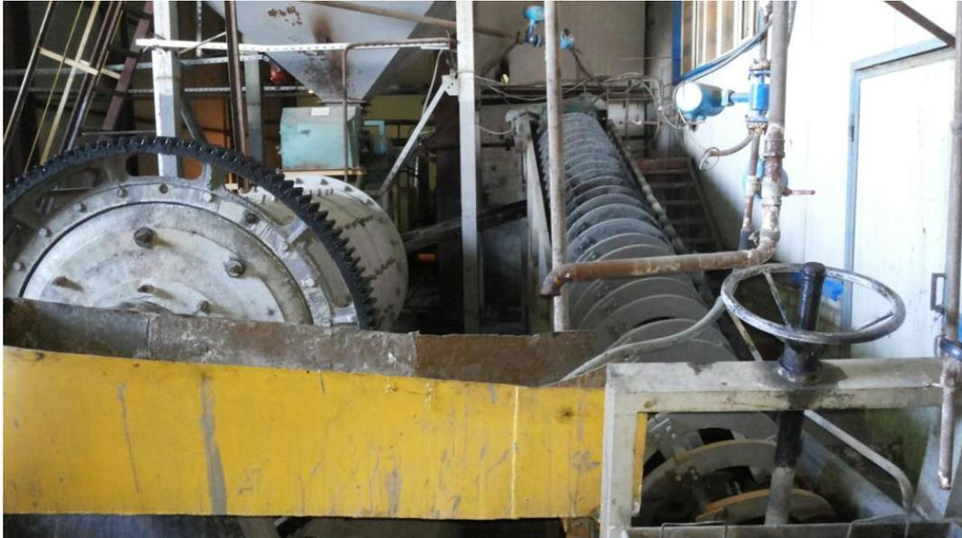
**Figure 7-2: Mill and Gravity Classifier**
